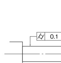
Space between two concentric cylinders with a radius difference of 0.1mm
