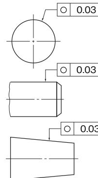
Space between two concentric circles with a radius difference of 0.03mm. Applicable to an arbitrary cross section perpendicular to the axis.
