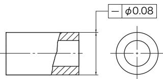
Space inside a cylinder with a diameter of 0.08mm
