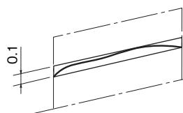
**Flatness** Flatness indicates the degree of deviation of a flat portion from the geometrical plane.
