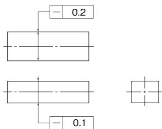
Space inside the prism enclosed by two pairs of parallel planes with intervals of 0.2mm and 0.1mm in the directions of indicated arrows
