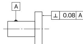
Space between two parallel planes with an interval of 0.08mm, perpendicular to the reference straight line
