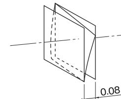
Perpendicularity of a flat portion with respect to the reference plane
