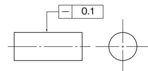
Space between a pair of parallel straight lines with an interval of 0.1mm on an arbitrary plane including the axis
