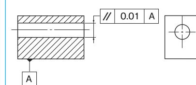
Space between two parallel planes with an interval of 0.01mm, parallel to the reference plane
