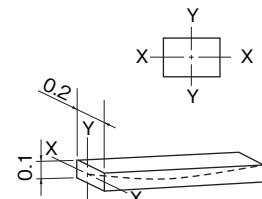
Straightness with no direction defined (Axis of a cylinder)
