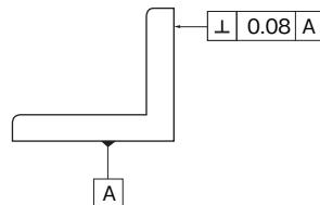
Space between two parallel planes with an interval of 0.08mm, perpendicular to the reference plane
